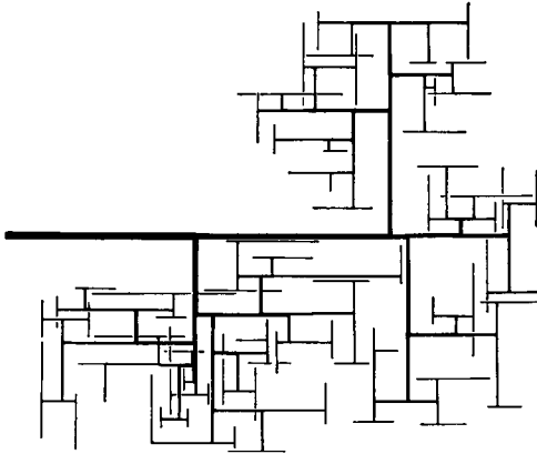
FIGURE 1 Diagram of an assembly with bifurcation to seventh order; the lengths of the branches are to scale, but the diameters are only indicated qualitatively. This assembly was the basis of all calculations except those shown in Figs. 7, 8, and 12.
